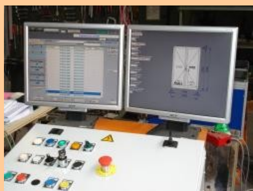
Control console equipped with a computer connected to the client's GPAO. The left screen lists the programs. The right screen displays the dimensions of the joinery being framed.
