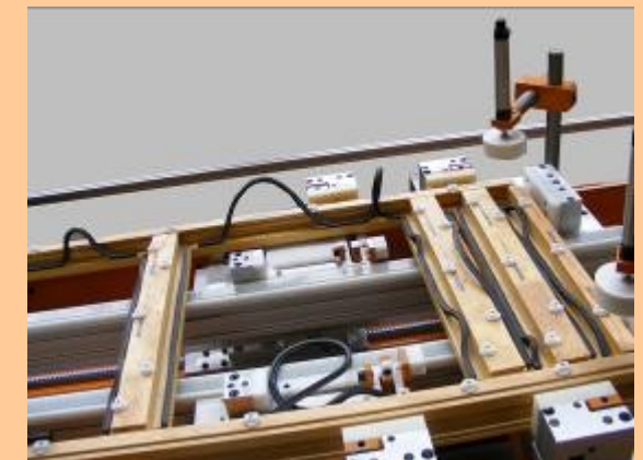
Example of joinery including an intermediate cross bar with 3 low cross bars forming a bottom rail.
