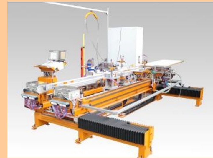
Horizontal framing screwing machine with in-line automatic evacuation of the joineries.
