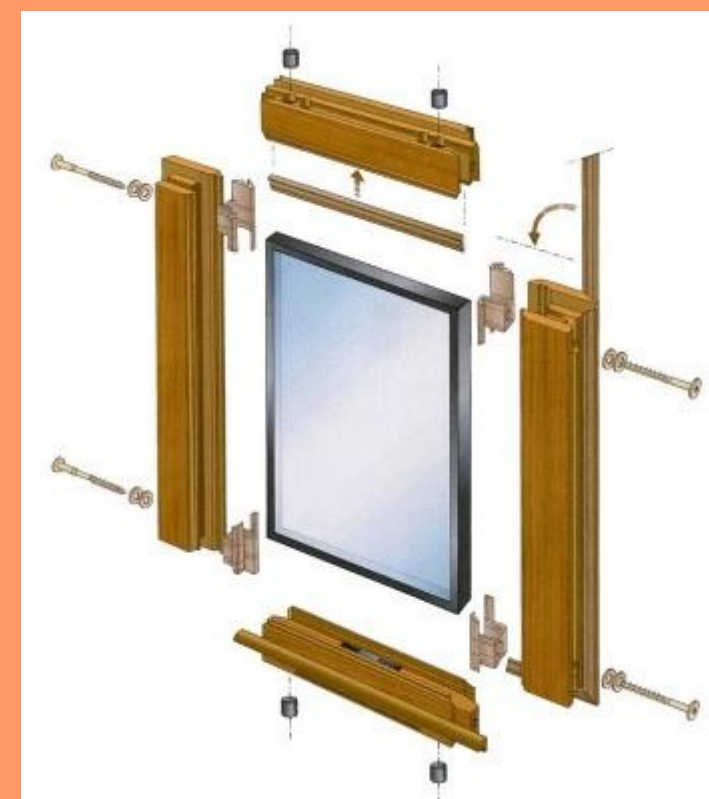
Example of mechanical assembled joinery using the inserted screw technique that renders the joinery detachable. A flawed part or the glass can be changed.
