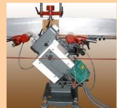
Special mortiser for square cutting
