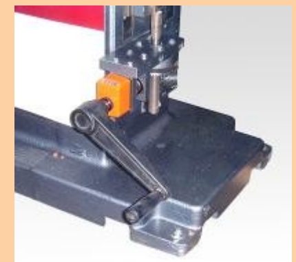
Ascending and descending system of the unit by a lever and mechanical numeric counter
