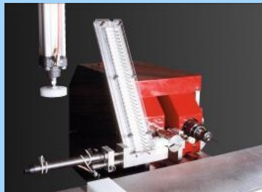
View of the entire hinge inserting unit, with the Anuba hinge magazine, the drilling unit and the digital rotation hinge inserting unit.
