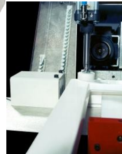
View from the reference thrust block with its part detecting cell.
