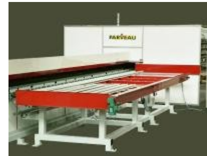
Loading storage unit
