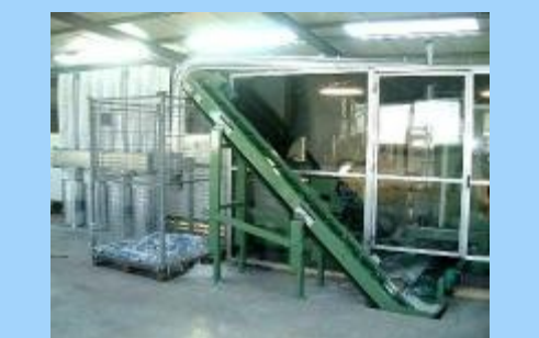
Conveyor belt and debris lift
