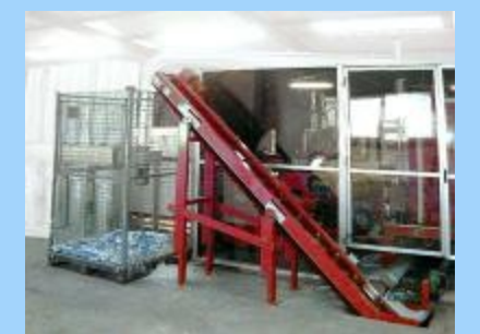
Conveyor belt for waste extraction (option)
