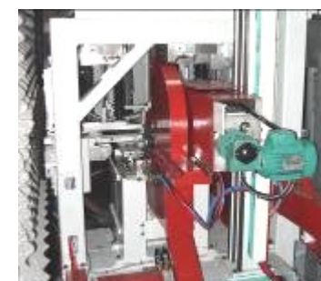
Sawing unit for cutting angles from - 45° to + 45°
