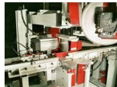
Sawing unit for 45° to 90° cut
